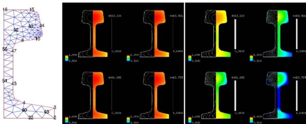
**Fig. 1** The domain  $\Omega$  is a half cross section of a rail profile. Different cost functionals (e.g. different output matrices) produce different final temperatures according to experimental observation.
