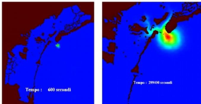
Figure 1.10: Concentration of a pollutant released in front of the Venice Lagoon at two different time steps.
